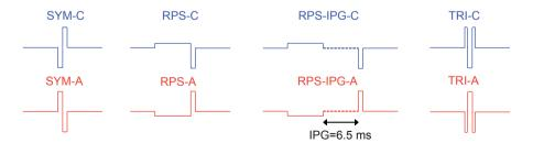
**Fig. 1** Schematic representation of the electrical pulse shapes used for stimulation, including symmetric biphasic cathodic-first (SYM-C) and anodic-first (SYM-A), Reversed pseudomonophasic with a short, high-amplitude cathodic (RPS-C) or anodic (RPS-A) phase, Reversed pseudomonophasic with a 6.5-ms interphase gap (RPS-IPG-C and RPS-IPG-A) and triphasic with a cathodic (TRI-C) or anodic (TRI-A) central phase
