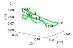
**Fig. 1.** Example of a manually segmented sub-trajectory from a mastoidectomy procedure containing 7 strokes. Units are in metres. Red crosses mark turning points and green dots mark normal points.
