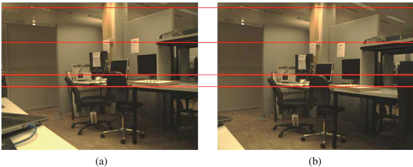
Fig. 29. Original images have distortions as observed on the lines (a) left image (b) right image.
