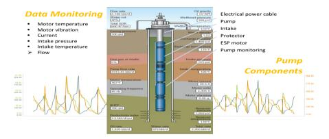
Fig. 1. Electric Submersible Pumps (ESPs)
