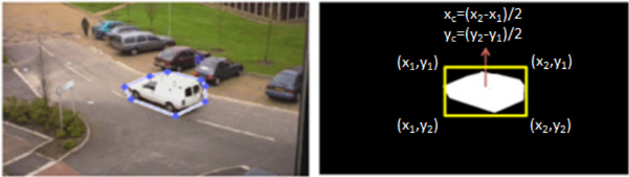
Fig. 2. Object selection and centroid extraction
