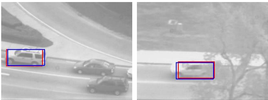
Fig. 2. Video sequence “car”; ground-truth box is displayed in blue color and tracking result in red; a) frame n.26 b) frame n.568
