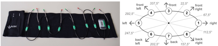
Fig. 3. The tactile belt with 8 vibrators (the interval angel of each vibrator is 45°)
