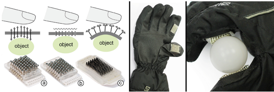
Fig. 4. (Left) The three different transfer mechanisms in the technology probes integrated into individual prototype gloves; (a) shape, (b) vibration and (c) lateral deformation. (Middle) Example of the glove prototypes: vibration transfer mechanism implemented on the index and thumb. (Right) The pins of the shape transfer mechanism deforming with the contour of a ball.
