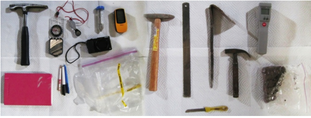
Fig. 3. Tools used by crew members during EVAs; ranging from geological hammers, spatulas, clinometer and thermometer, to pens, GPS and camera.
