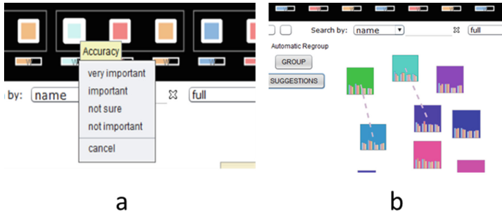
Fig. 2. Knowledge collection interfaces of MindMiner. a: Interface for active polling with uncertainty . b: Interface for example-based constraints collection .
