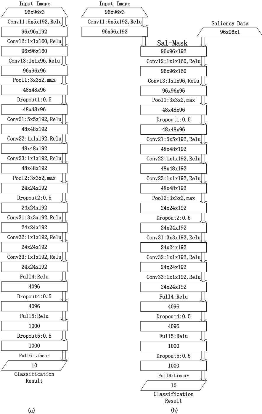
Fig. 5. Structure of NIN and Sal-Mask Network deride from it. (a) is NIN, (b) is the Sal-Mask Network derided from NIN.
