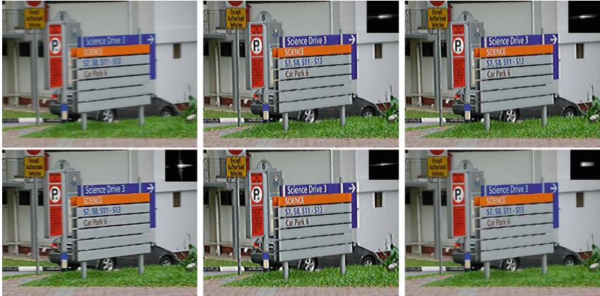
Fig. 2. Blind motion deblurring with the real-world example (image size: 640 \times 480 , kernel size: 21 \times 21 ). From left to right, top to bottom: blurred image, deblurred images with estimated blur kernel by Cho et al. [2], Xu and Jia [3], Krishnan et al. [5], Xu et al. [6] and the proposed approach.
