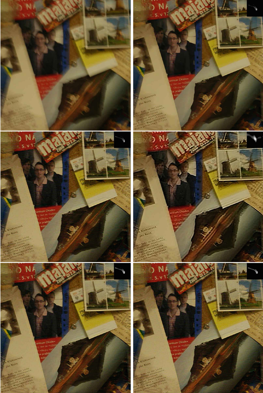
Fig. 3. Blind motion deblurring with the real-world example (image size: 800 \times 800 , kernel size: 51 \times 51 ). From left to right, top to bottom: blurred image, deblurred images with estimated blur kernel by Cho et al. [2], Xu and Jia [3], Krishnan et al. [5], Xu et al. [6] and the proposed approach.
