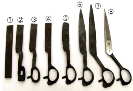
Fig. 1. Photo of the eight steps for manufacturing sewing scissors.
