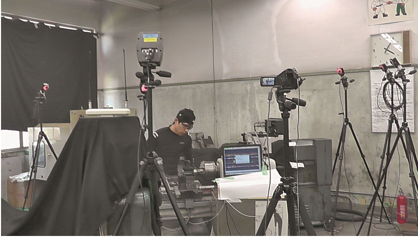
Fig. 6. The experiment setup for recording the motion of chucking movement and muscular activity.
