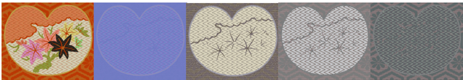
Fig. 10. Part of the BTF textures of Noh costume. From left, diffuse map, normal map, specular map, \sigma_x map, and \sigma_y map.
