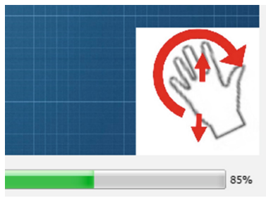
Fig. 6. Icon and progress bar into SMA to show state of interaction using Leap Motion device.
