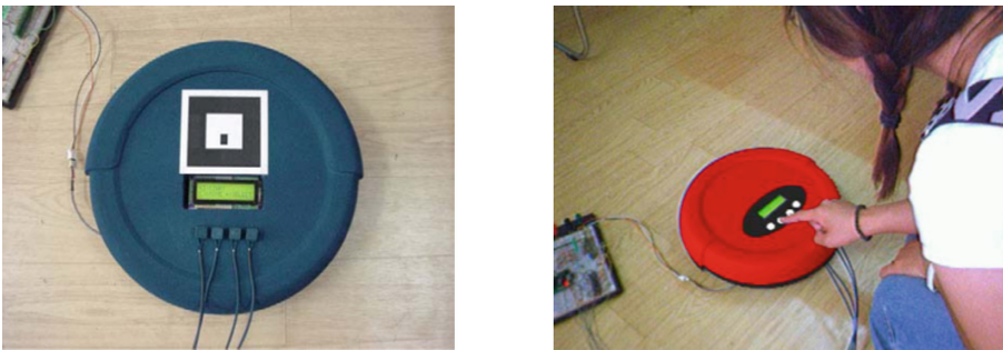
Fig. 3. Physical artifact of a cleaning robot (left) equipped with a marker to enable a tangible augmented view (right) with natural interaction.
