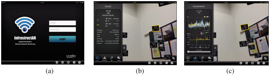
Fig. 3. InfrastructAR, an AR application designed to help the Georgia Tech community understand how the hidden WiFi infrastructure works. (a) shows the login screen based on Georgia Tech’s web-based authentication system, (b) shows the details of the access point, and (c) is a real-time visualization of the network traffic flowing through that access point.
