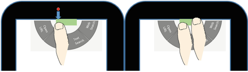
Fig. 3. Holding a virtual clipboard by swiping from the bezel to the clipboard and then tapping the clipboard with another finger.
