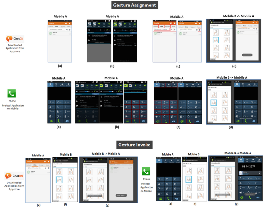
Fig. 9. GESTURE ASSIGN (a) Open Target Screen (b) Drop down notification bar and select bend register (c) Highlight selectable widgets and select target widget (d) Select bend type from bend emulator and assign gesture on demo prototype. GESTURE INVOKE (e) optionally open the desired screen (f) Select bend type from ‘Bend gesture emulator’ (g) This triggers the action registered on the target widget (Delete chat action for ChatON& Last call action for Dialer).
