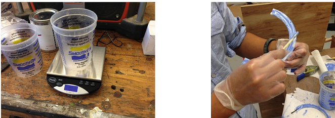
Fig. 7. The picture on the left demonstrates how the silicone was measured on the scale. The picture on the right shows the process of filling the 3D printed mold.
