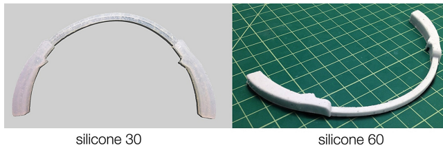
Fig. 1. It shows the difference between the silicone 30 and silicone 60. Silicone 30 is too soft to stay on users' neck.
