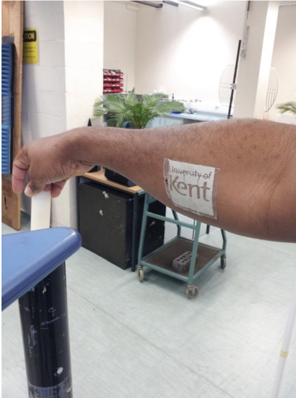
Fig. 8. Read range measurement of Kent logo tag
