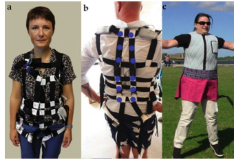
Fig. 2. a. Inner Layer Adjustable Harness Front. b. Inner Layer Harness Back. Blue dots indicate actuator positions for up and down patterns. c. Outer padded stretchable vest and skirt
