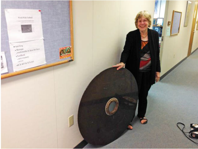
Fig. 1. A 48 inch computer disk from the BCC 500 computer
