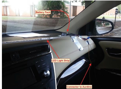
Fig. 3. Adafruit NeoPixel digital RGB LED strips light set up (Color figure online)
