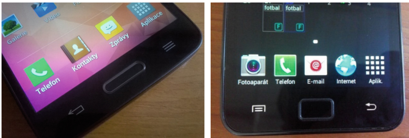
Fig. 2. LG cell phone (left) and Samsung cell phone (right). Note the opposite mapping principle represented by the position of the “back” button.
