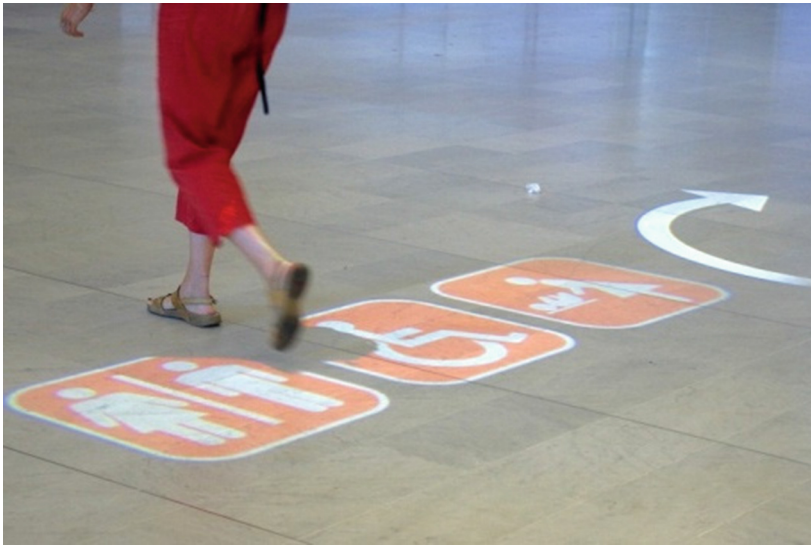
Fig. 7. Paris, France, 2013. A smart solution of a complicated wayfinding situation at Paris CDG Airport uses a projection on the floor immediately after stepping out of the escalators, combined with an animated arrow suggesting the direction of walk.
