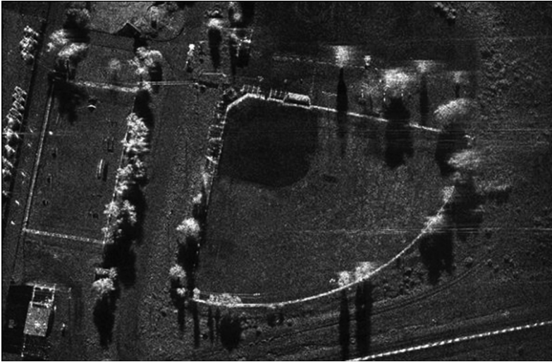
Fig. 1. SAR image of a baseball diamond. Image courtesy of Sandia National Laboratories, Airborne ISR.
