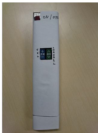
Fig. 2. Most basic television remote controller for casual users of consumer electronics.
