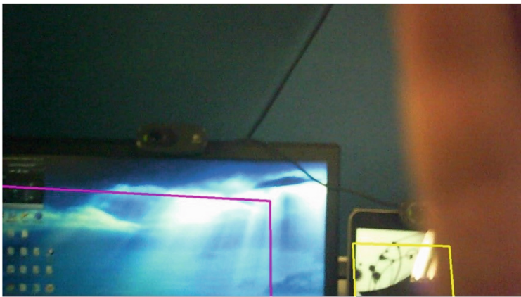
(c) Actual image taken by the camera on the eyeglass superimposed by the estimated appearances of the devices.
