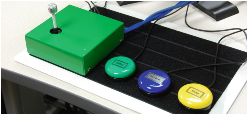
Fig. 1. The Smart Voting Joystick with Enter, Review, and Help buttons
