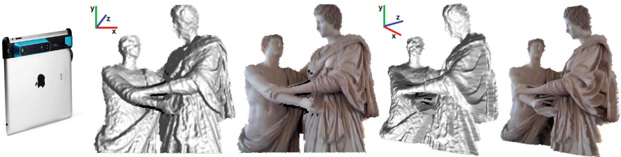
Fig. 1. Example of an RGB-D frame captured by the camera and depth sensor for a tablet computer (shown on the left). The same depth frame is rendered from two different perspectives —with and without color texture. Images shown with permission from the Italian Ministry of heritage, cultural activities and tourism. Su concessione del Ministero dei beni e delle attività culturali e del turismo - Soprintendenza Speciale per il Colosseo, il Museo Nazionale Romano e l’area archeologica di Roma.
