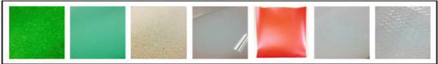
Fig. 1. Sample materials for Exp.1 (from the left, Grass mat, E.V.A., Cork, Acryl, Rubber, Cotton, and Air cap).
