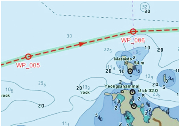
Fig. 4. The ship has sent the route to the STCC and got it back as a “recommended” route. Accepting the route then makes it an agreed, “green” route, signifying that this route will be used for coordination with other ships’ routes (Color figure online).
