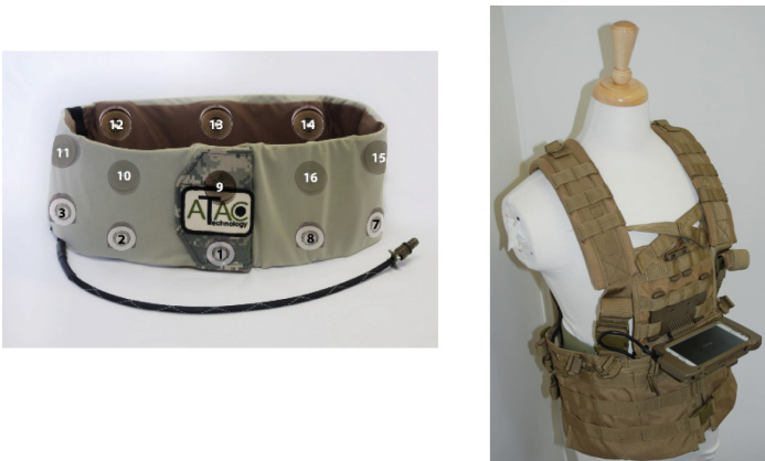
Fig. 1. NavCom tactile belt showing tactor placement (left) and chest-mounted visual display (right).
