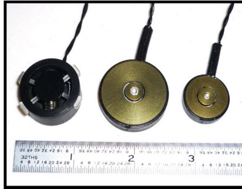
Fig. 2. The EAI EMR, C-2, and C-3 tactor transducers (left to right respectively)
