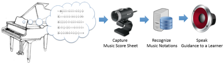
Fig. 1. Overview of musical score recognition process to give hints to music learners
