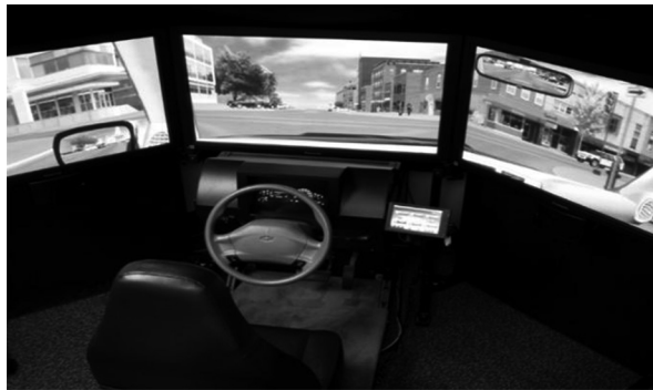
Fig. 1. After affect induction procedure, all participants drove the same predefined route that includes hazardous events, using the NADS MiniSim.
