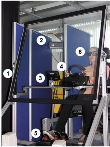
Fig. 1. Experimental setup with components and a test participant with laser safety glasses (6)
