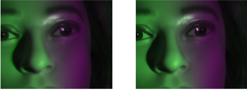
Fig. 3. Registration of camera frames I_1^c (green colour channel) and I_3^c (magenta colour channel) belonging to the same frame sequence. Left: before registration. Right: after registration. The misalignment is most easily seen at the edge of the iris and corners of the eye.
