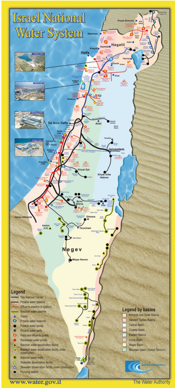
Fig. 16.2 Israel national water system (Source: Israel Water Authority)
