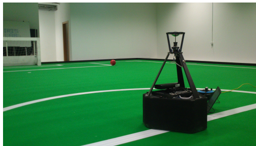
Fig. 9. Example of kinect calibration set-up with a ball on a well known position.
