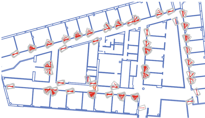
Fig. 9. The most commonly observed object, doors, as discovered by Model-Instance Object Mapping. Our algorithm correctly detected all the doors in the environment without any supervision.
