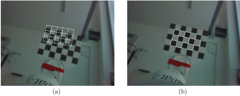
Fig. 5. The checkerboard projection without calibration (a). The resulting projection with optimized parameters \alpha (b).
