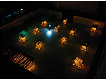
(a) Field with illuminated obstacles where the robot has to find objects in the dark with just a headlight.
