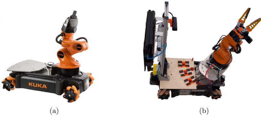
Fig. 1. (a) Stock youBot. (b) smARTLab@Work modified youBot for world championships 2014.
