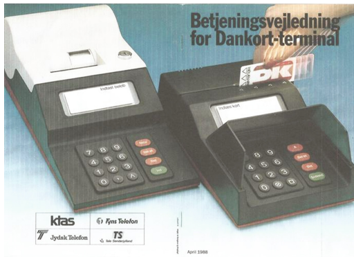
Fig. 2. The Dankort terminal. To the left the shop cashier’s terminal, where she entered the amount and printed the receipt. To the right the customer terminal with card reader and key-board for the PIN-code.
