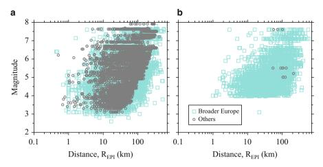
**Fig. 12.5** Magnitude and distance distributions of **(a)** SHARE and **(b)** EMME strong-motion databases. The SHARE accelerograms from the broader Europe are shown in cyan to give a more clear view on the fraction of recordings from this region in the SHARE database. Same color codes are used in the EMME scatter plot to compare the strong-motion data distribution of broader Europe between these two databases
