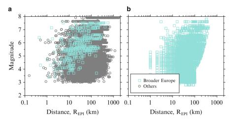
**Fig. 12.6** Comparison of (a) NGA-West2 and (b) RESORCE strong-motion databases in terms of magnitude and distance distribution. The NGA-West 2 database contains 21,336 strong-motion recordings and only 2 % of the data is from the pan-European region. The colored data given on the scatter plot of NGA-West2 show the pan-European accelerograms in this database
