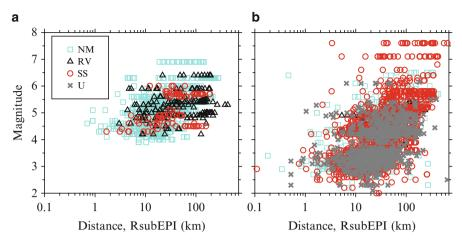
**Fig. 12.4** Magnitude vs. distance scatters of (**a**) ITACA and (**b**) T-NSMP databases. The ITACA<sup>5</sup> project compiled a total of 2,182 accelerograms from 1,004 events (Luzi et al. 2008) whereas T-NSMP studied 4,607 strong-motion records from 2,996 earthquakes recorded at 209 stations (Akkar et al. 2010). The symbols on the scatter plots show the distribution of fault mechanism in each database (Refer to the caption of Fig. 12.3 for abbreviations in the legends)
