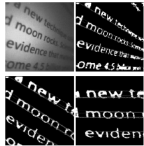
Fig. 3. A demonstration of our perspective and rotation correction algorithm.
