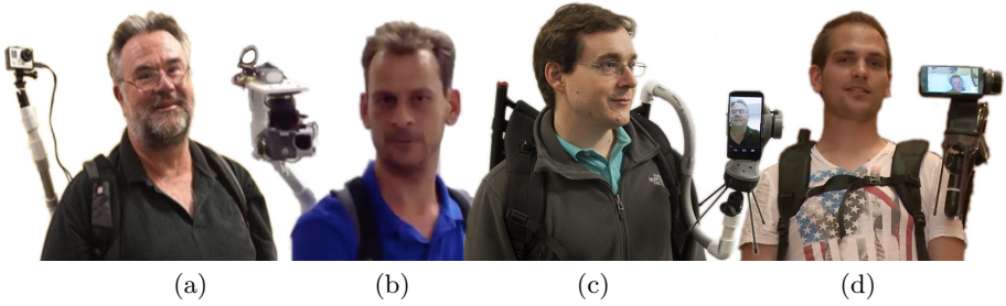
Fig. 2. Polly Prototypes: (a) first frame mounted version, (b) first stabilized version, (c) portrait phone, (d) current landscape version
