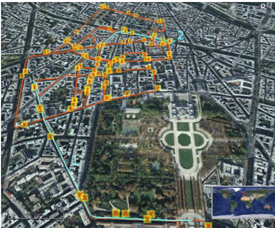
Fig. 5. Road sign landmarks (yellow squares) and vehicle trajectories overlapped on Google Earth. The reference data sequence used for generating the landmarks database is shown in orange; the two test trajectories are shown in cyan.
