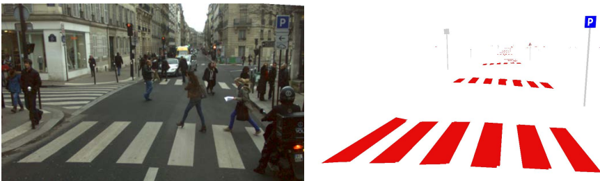
Fig. 2. (Left) One of the real images used for database generation; (Right) Reconstructed 3D road signs and road marking strips in the database
