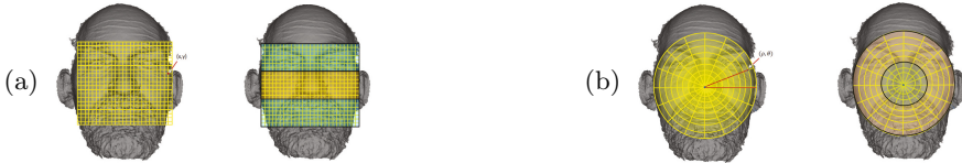
Fig. 2. (a) Global and local rectangular control grid in Cartesian coordinates; (b) Global circular and local annular control grid in polar coordinates
