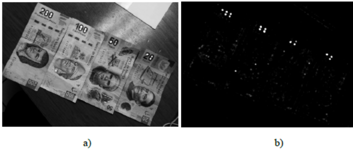
Fig. 3. Detection of semicircular regions corresponding to the denomination of banknotes via the FRS transform. a) Test image on which the maxima of the FRS transform has been overlaid. Image contrast has been exaggerated for illustrative purposes. b) Accumulator of the FRS transform; local maxima appear as bright spots. Notice that besides the desired maxima corresponding to banknote denomination numbers, some spurious maxima also appear.
